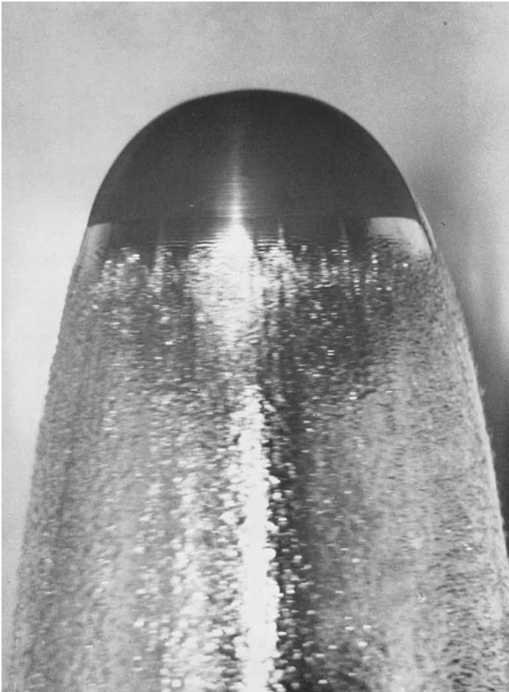
FIGURE 4. Microflash photograph of ventilated cavity at U = 30 ft./sec, \sigma = 0.127 .
